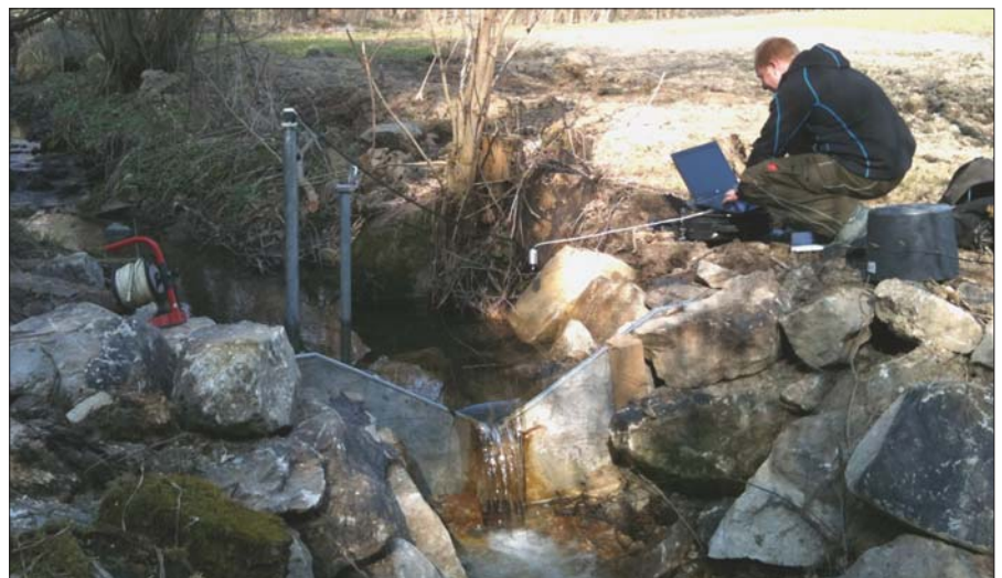
Flow measuring weir with automatic data collector
