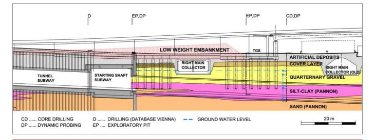
Excerpt of a longitudinal subsoil profile in the area of the subway crossing
